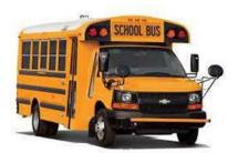
**Type "A" School Bus** - is a conversion or body constructed utilizing a cutaway front-section vehicle with a left side driver's door and a gross vehicle weight rating (GVWR) of 21,500 pounds or less.
