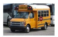
Type "A" School Bus – a conversion or a body constructed utilizing a cutaway front-section vehicle with a left side driver's door and a gross vehicle rating (GVWR) or 21,500 pounds or less
