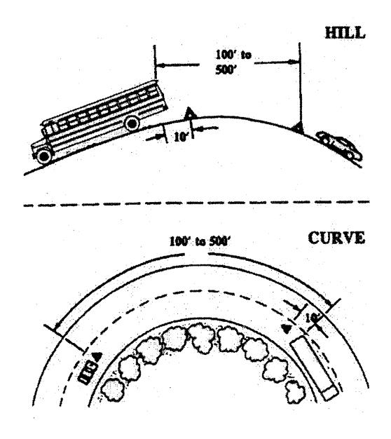
Reminder: If the line of sight is obstructed due to a hill or curve, move the rearmost triangle to a point giving adequate warning.
