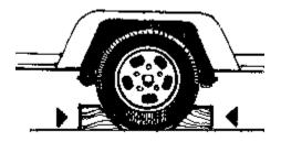
Whenever the trailer is detached from the tow vehicle, block the wheels so it is impossible for the trailer to roll off on its own. Better yet, do not ever detach the trailer on any grade.
