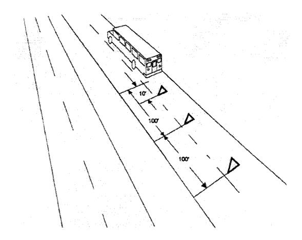
When placing the triangles, hold an assembled triangle toward the oncoming traffic. This enhances safety by increasing visibility to other drivers (especially at night).
