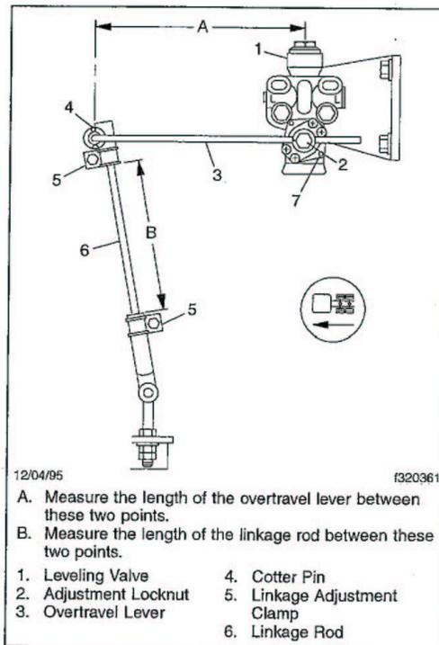
**Fig. 2, Overtravel Lever and Linkage Rod Measurement**
