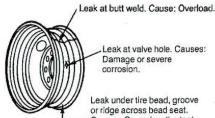
Leak at butt weld. Cause: Overload.
