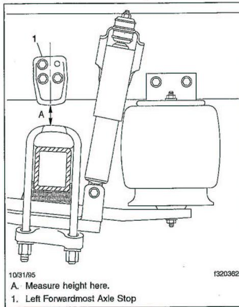
Fig. 3, Axle Stop Measurement
