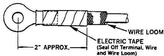
**Typical wire ending when replacing damaged wires or corroded terminals.**
