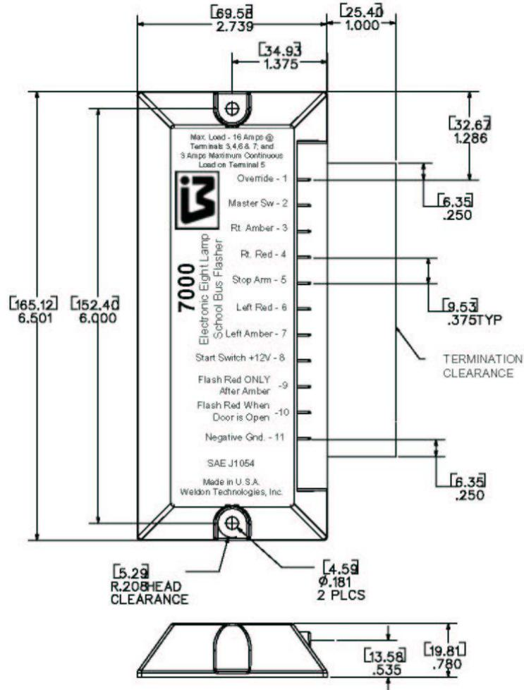
Figure 1 – Flasher Installation Drawing
