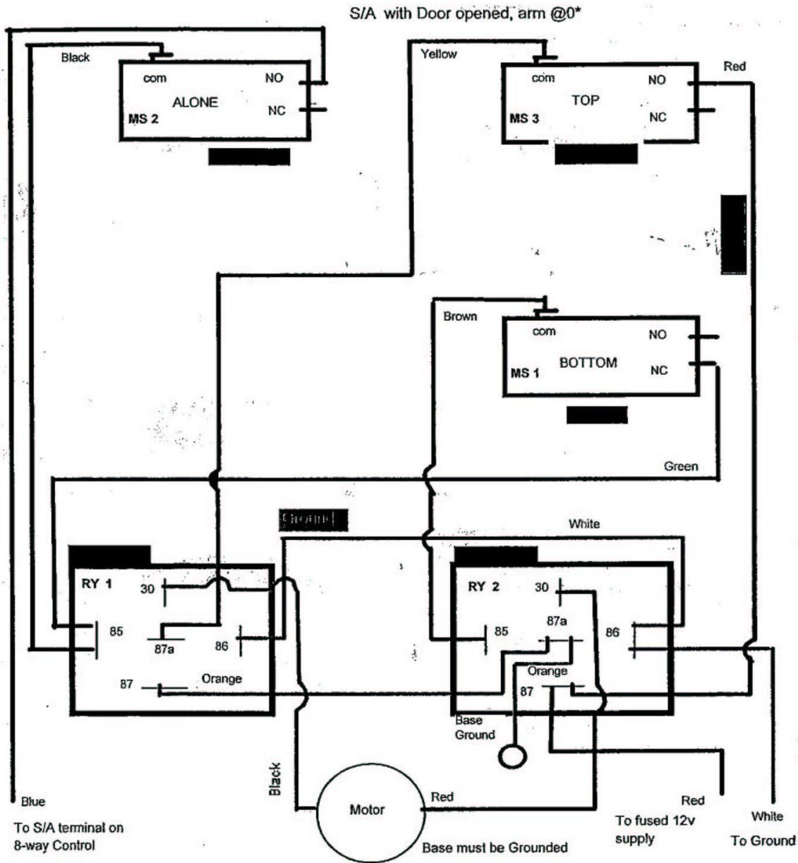
When the door is opened, the Blue wire from the 8-way Control becomes a steady 12v signal. This signal energizes both relays which reverses the voltage polarity on the motor leads resulting in the motor running to  $\pm$ open/E the arm to the 90\* position as determined by MS1 and the cam!
