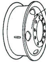
Cracks at disc nave
