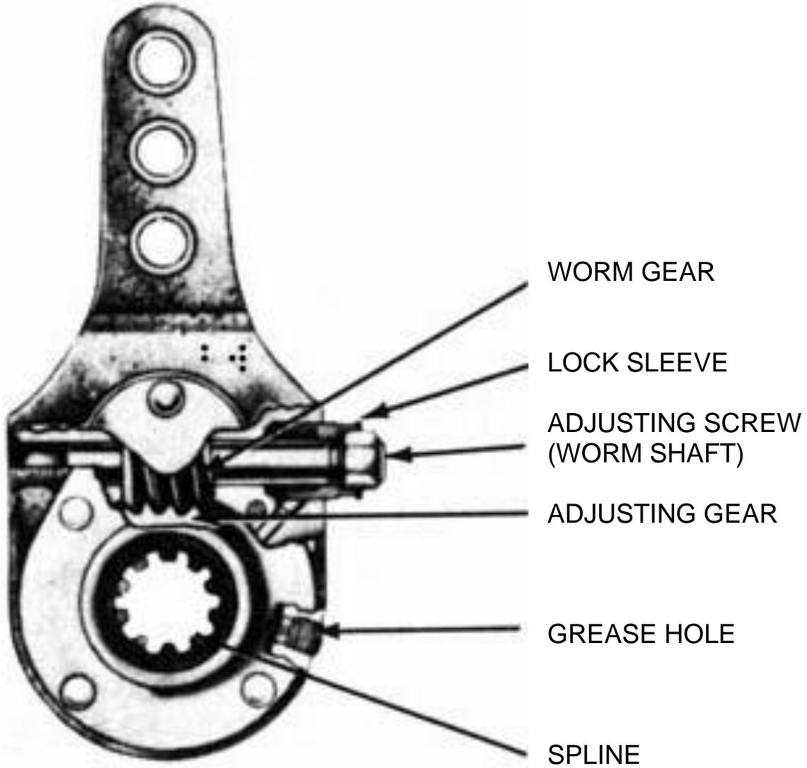
The slack adjuster should be adjusted with the threaded clevis or yoke and the adjuster screw, so that the brake chamber push rod is at a 90 degree angle with the slack adjuster arm in the brake full applied position. Then, consult the data chart for specifications on the particular type brake chamber in question.
